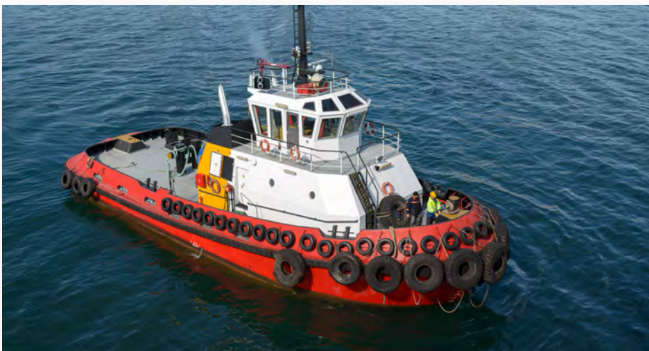
Articulated tug barges utilize PTMS Chargers to maintain batteries and supply power to essential services
