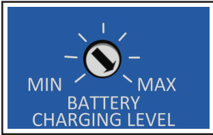
Figure 11: Current Limit/Battery Charge Level - Dial
