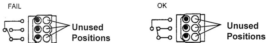
FIGURE 6: “FAIL” AND “OK” RELAY CONTACT POSITIONS
