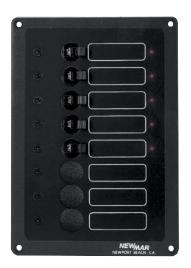
**ACCY-IX:** 8 breaker capacity, 5 installed standard; 2-5A, 1-10A, 1-15A, 1-20A or specify. 8 DC circuit "ON" indicator lights installed standard, AC lights optional. Size: 7 1/2" x 5 1/4", Weight: 2 lbs.
