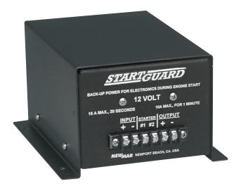
StartGuard solves this problem by providing supplemental voltage to sensitive electronics while the engine is cranked. It contains a sealed rechargeable battery which is switched online to electronics when the starter switch or solenoid is engaged. When the engine is running StartGuard automatically goes offline and the internal battery is recharged by the alternator.
