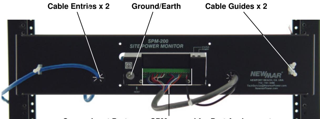
Sensor Input Ports, see SPM manual for Port Assignments
